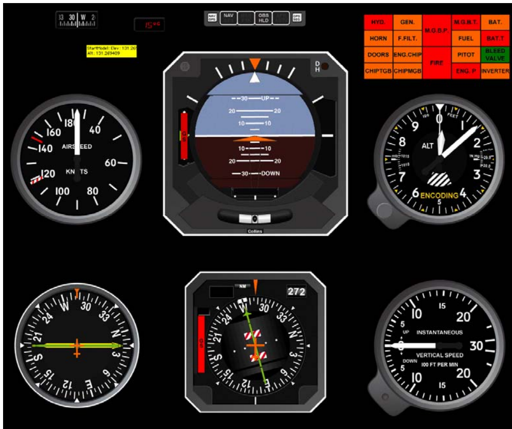
S623 Helicopter AATD Pilot Instrument Panel with Master Caution Panel
