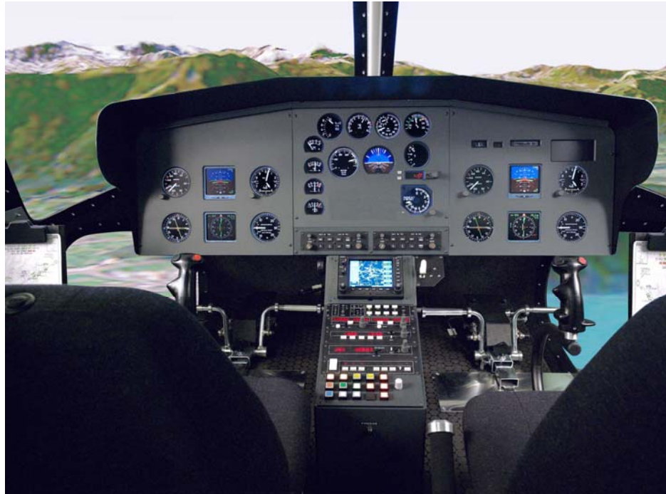
S623 Instrument Panel with GNS 430 GPS and Dual EFS-40 (EFIS)
