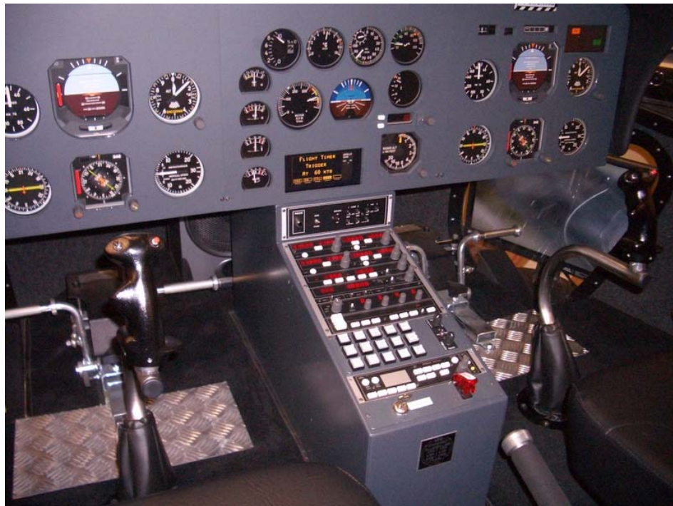
S623 Instrument Panel with Apollo GPS and HSI / RMI
