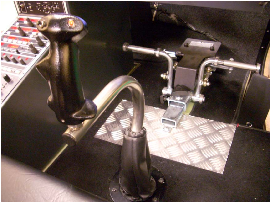
S623 Cyclic and adjustable anti-torque pedals
