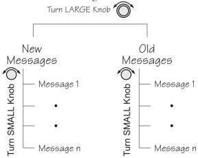
While any old message exists, the MSG annunciator remains steadily on at all times unless new messages arrive or all old message conditions go away.
