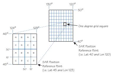
If you want to fly to the Bravo-Charlie 3 corner of the 45°N and 123°W grid, you would define the corner as a USER waypoint with the name "53BC3." The SAR position is set to 40°N and 120°W.
