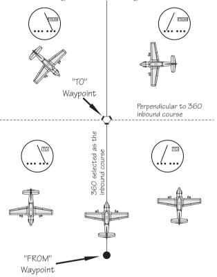
When you are ready to depart the hold, you enable sequencing with the OBS/HLD button. If you are on the "TO" side of the waypoint, the flight plan will sequence the next time you cross the waypoint. If you are on the "FROM" side of the waypoint, the flight plan will sequence immediately. The following example shows holding at the Newburg VOR (UBG) with  $020^{\circ}$  inbound selected as the "OBS" course to UBG.
