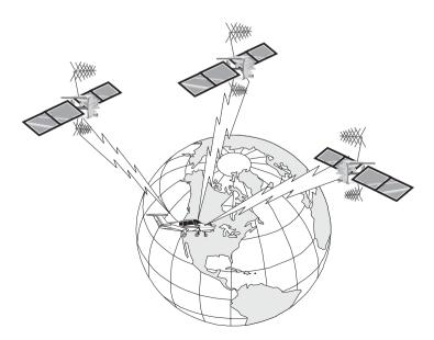
processes the information to determine which satellites are "visible" to the receiver's antenna. With this determination made, the receiver chooses satellites to calculate a position fix. Using information transmitted from three or more satellites, the unit can calculate latitude and longitude (usually abbreviated Lat/Lon); with four or more satellites, GPS altitude can also be calculated.
