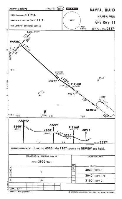
Approach Example 1 -Straight In This example illustrates the approach to Nampa, Idaho. This example was selected because it is a new approach designed especially for TSO C-129 GPS equipment. It is probably as simple an approach to fly with the Apollo GX as there is.
