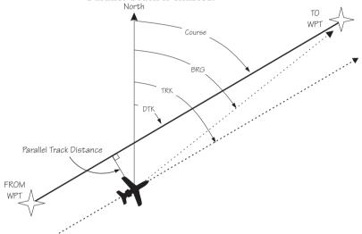
When Parallel Track is selected, the course line drawn on the Map pages will show the parallel course. If the Hold function is used when Parallel Track is selected, the Hold waypoint will be the phantom waypoint on the parallel offset, not the actual waypoint. Using Direct-To, loading an approach, or editing your flight plan will automatically cancel Parallel Track. A series of turns, even if less than 120°, is not allowed if the "inside" parallel tracks would overlap.
