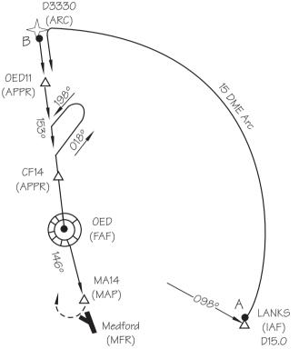
Create a flight plan from Klamath Falls, Oregon to Medford, Oregon. Activate the flight plan and then load an approach. Select the VOR DME 14: LANKS approach. The main approach waypoints are shown in the list; intermediate points are not.
