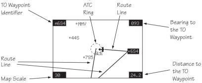
1. In the Map function, turn the LARGE knob to reach the Map Setup page. Press SEL to start selection of the Route Line. The Route Line selection will flash. Or, press the RTE smart key to toggle through the choices.
