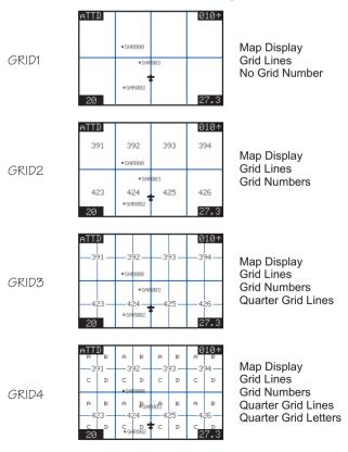
**Basic Grid Type** GRD – No grid lines GRD 1 – 60 minute grid lines GRD 2 – 30 minute grid lines
