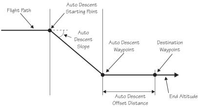
Each time you begin to edit the Auto Descent values, the End Altitude is automatically reset to 1,000 feet over the altitude of the desired Auto Descent Waypoint, if the waypoint is an airport. Otherwise, the End Altitude automatically resets to 2,000 feet. In addition, the default Auto Descent Waypoint is automatically updated, as long as Auto Descent is OFF, to the current TO waypoint each time a waypoint sequence occurs. Set up your Auto-Descent by selecting:
