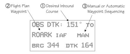
Selection of automatic or manual sequencing is only available after an approach is enabled. Entering a desired inbound course to a waypoint automatically suspends leg-sequencing at that waypoint and lights the **OBS/HLD** annunciator.
