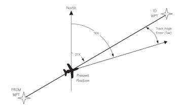
**Track Angle:** The angle of your actual direction of travel. Track angle is computed using the magnetic variation at the Present Position.
