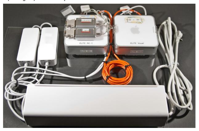
Two Mac Mini computers are mounted onto the plexiglass, a main computer labeled "ELITE RC-1" which powers the simulator, and a visual computer labeled "ELITE Visual" which powers the visual. Out of the box, they should already be connected to their power adapters, which are also mounted in place, and plugged into the surge protector. The computers are also connected together by a CAT-6 crossover network cable, which allows them to communicate with each other.
