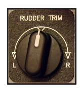
The RUDDER TRIM knob allows the operator to trim off rudder pressure caused by asymmetric power or drag. The RUDDER TRIM knob should be in the top center position for normal operations.
