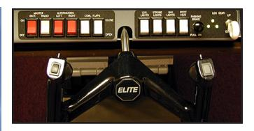
The sub panel located to the *left of the yoke* contains six rocker switches. The first four from the left are for the Battery, Radio Master and Alternators respectively. The up position is ON and the down position is OFF. The two switches on the right control the Cowl Flaps. The up position closes the cowl flaps while the down position opens the cowl flaps.
