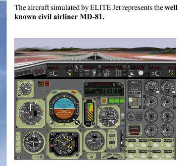
The instrumentation of the cockpit represents all standard instruments. Only the captain's side of the cockpit is represented for the navigation instruments. In a real cockpit, the same navigation and flight instruments are installed on each side.
