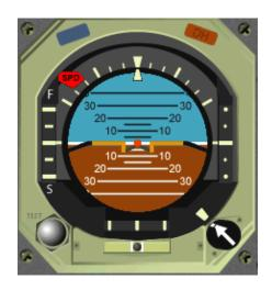
The Attitude Director Indicator (ADI) is the most important instrument in the cockpit for instrument flying. ELITE Jet has a standard ADI. For attitude reference, an integrated scale is provided with a mark every 5° through the first 20° and a larger mark and degree indication every other 10° through 40°. This scale represents the aircraft nose up (ANU) or aircraft nose down (AND). At the top of the ADI there is a small yellow triangle called the skypointer that is used for bank angle reference.
