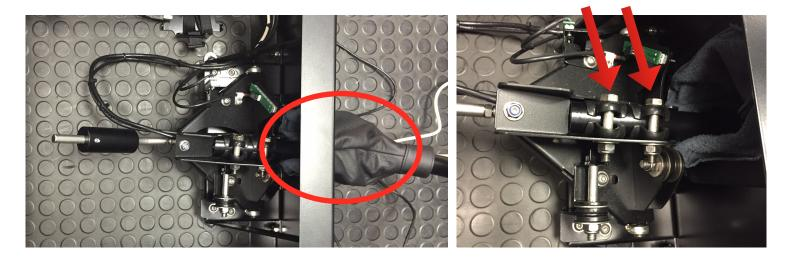
2. Attach the metal brackets to the seat by first removing the bolts (shown below) then with the seat brackets in place replace them to the same holes and tighten the seat in place.
